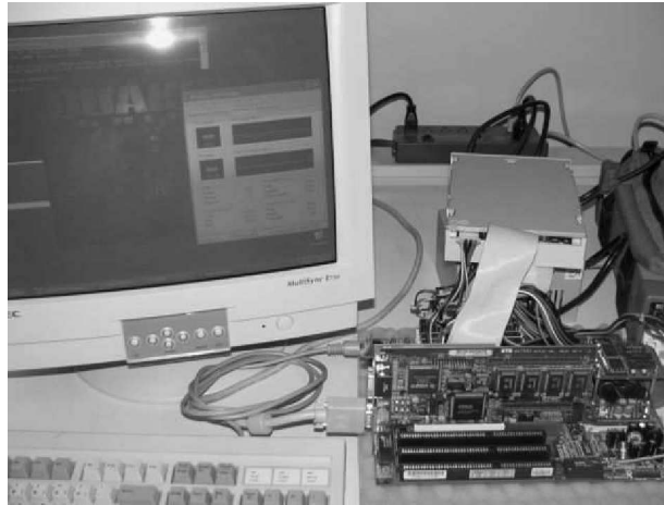
Fig. 1. Image of the FPGA-based processor emulator system equipped with standard hardware peripherals, a Xilinx Virtex-4 device in place of a microprocessor chip, all running Windows XP.
